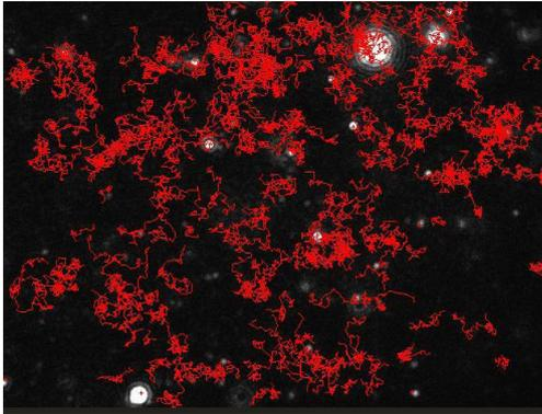
NanoSight's nanoparticle tracking analysis uses Brownian motion to locate and follow individual particles in solution.
