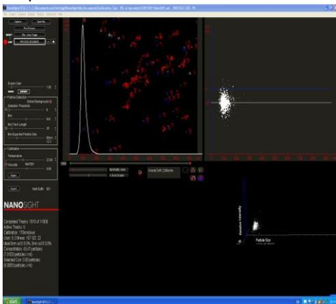
NTA analysis of a recorded video after the electro-osmotic profile has been characterised. The scatter plot in the top right shows corrected electrophoretic velocities in white, plotted against particle size. Velocities are converted into zeta potential measurements by scaling according to sample properties.
