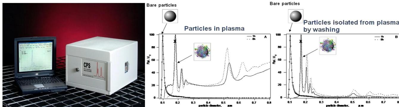
DCS equipment, and example of determination of the effective size of nanoparticles in the absence (bare) and presence (corona) of human plasma. The corona is very similar *in situ* and following washing to remove the loosely bound proteins.
