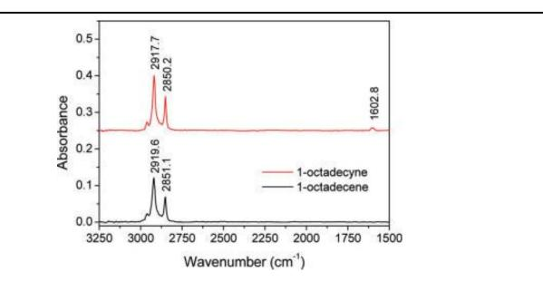
Part IR spectrum of an ATR measurement of monolayers (Luc Scheres, Marcel Giesbers and Han Zuilhof, Langmuir, **2010**, *26* (7), pp 4790–4795) Clearly visible are the C-H stretch vibration of the aliphatic chain and in the case of the attached alkyn the remaining C=C stretch vibration.
